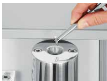
Feeding the sample to the furnace
