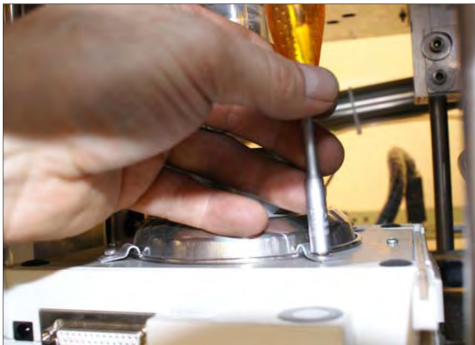
Fig. 3.8.6: LHS/RHS – Loosen the balance shield
