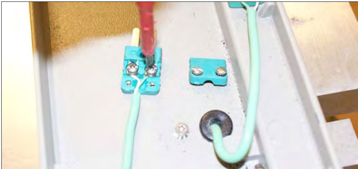
Fig. 3.9.3: TS – Disconnecting cable from the plug
