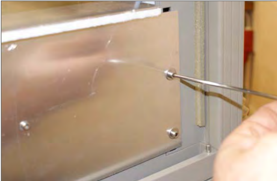
Fig. 3.9.4: RHS – Unscrewing isolation plate
