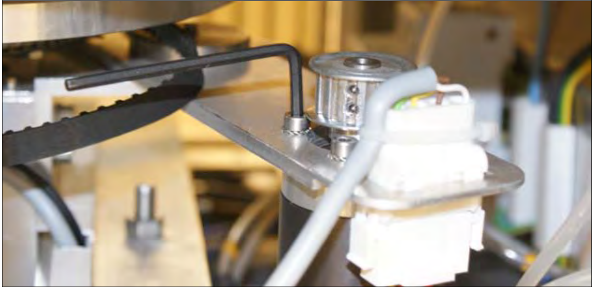
Fig. 3.10.4: RHS – Unscrewing the screws holding the motor
