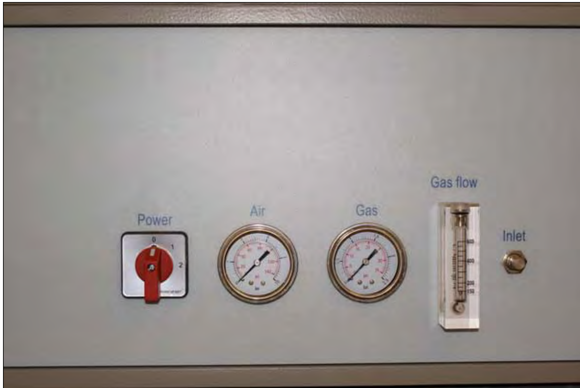
Fig. 2.2: FS – Front with manometers and flowmeter
