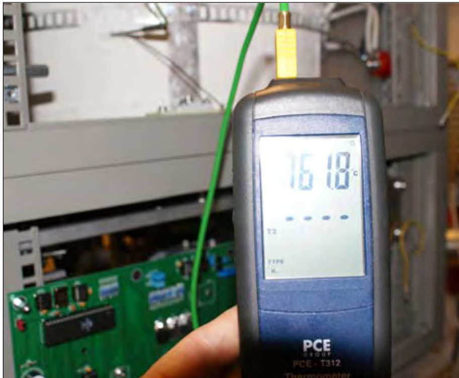
Fig. 3.1.2: External measurement of furnace temperature during analysis
