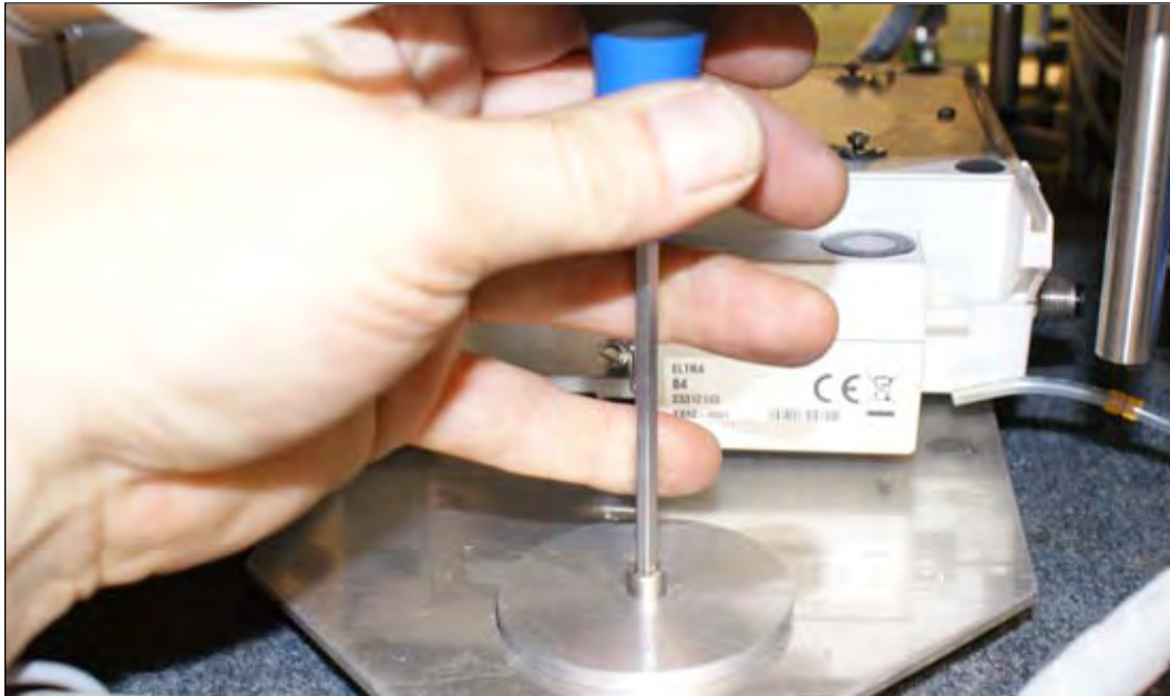
Fig. 3.8.7: LHS – Unscrew balance base plate
