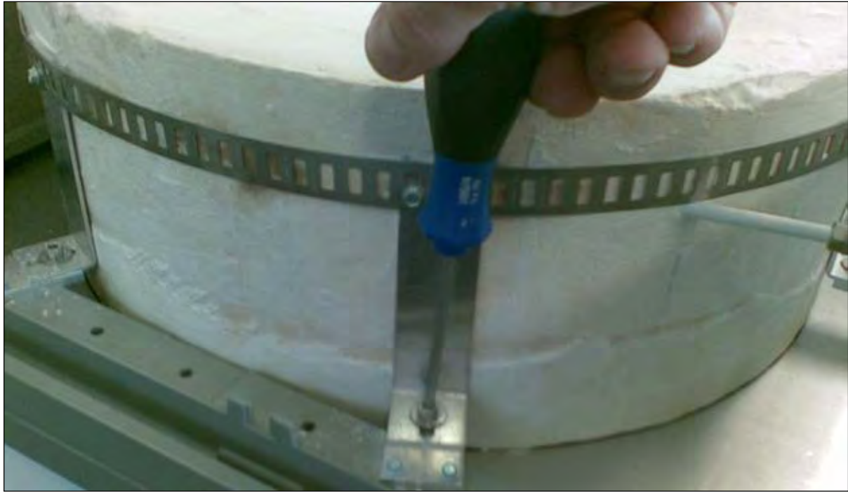
Fig. 3.16.7: Loosing the front positioning supports of upper heating element
