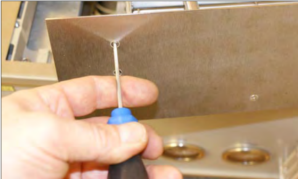
Fig. 3.6.3: FI – Cover of internal blower
