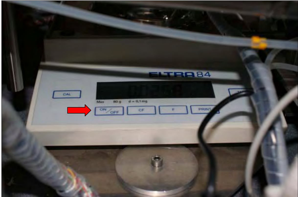
Fig. 2.4: RHS – Balance display and -operation elements
