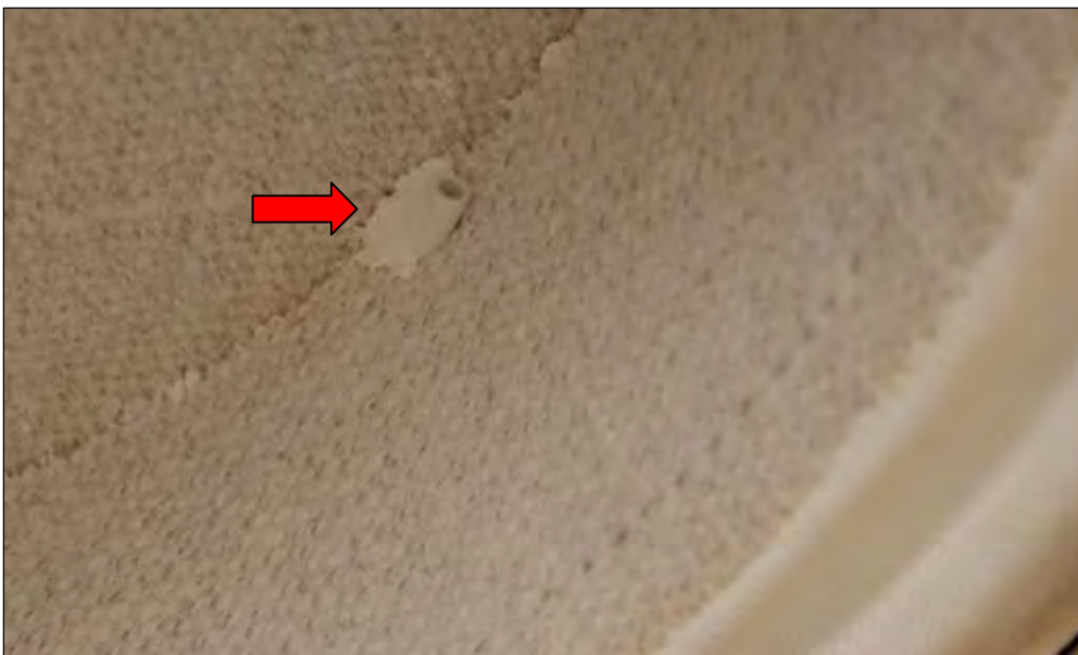
Fig. 1.7: FI – Purging port at the upper heating element
