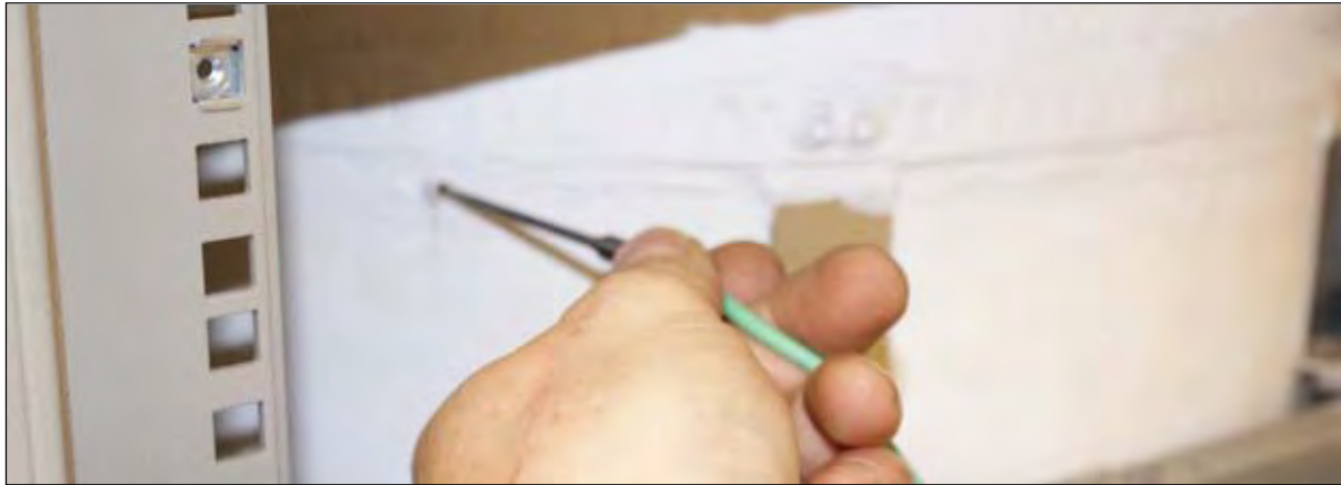
Fig. 3.9.6.: RHS – Removing of the Thermocouple out of the ceramic tube
