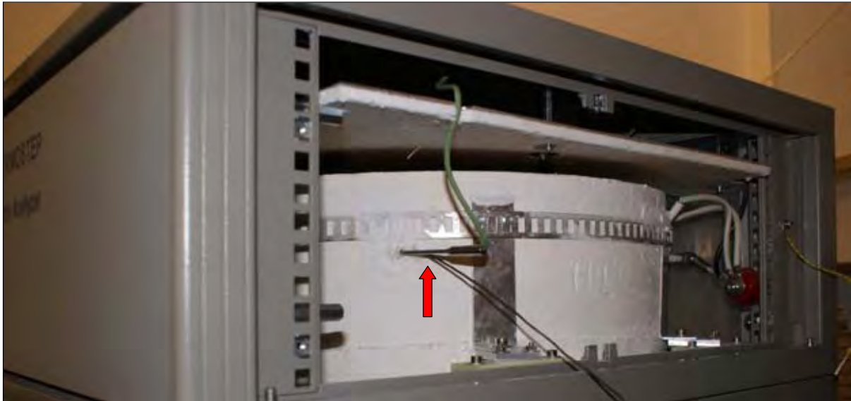
Fig. 3.1.1: RHS – Removed left, upper side panel and isolation plate (red arrow: external thermocouple)
