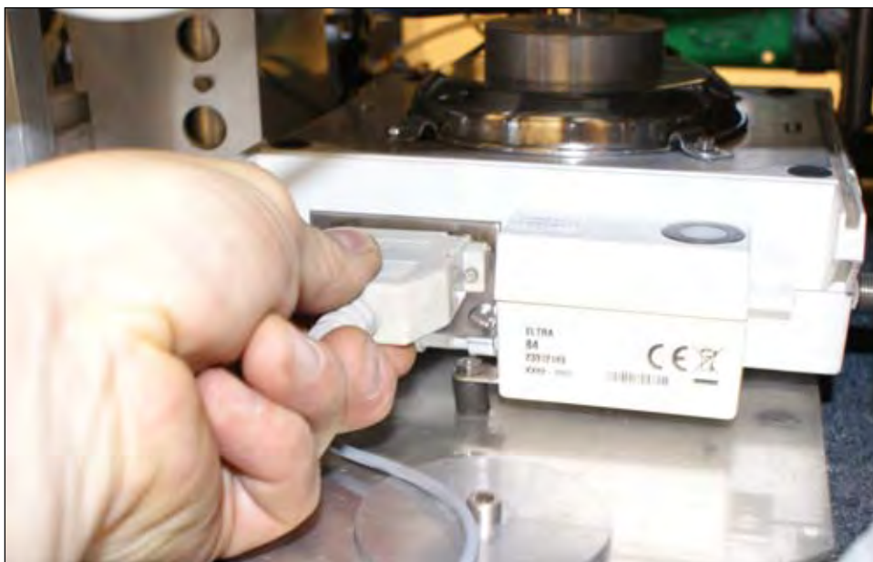
Fig. 3.8.4: LHS – Unplugging balance cable
