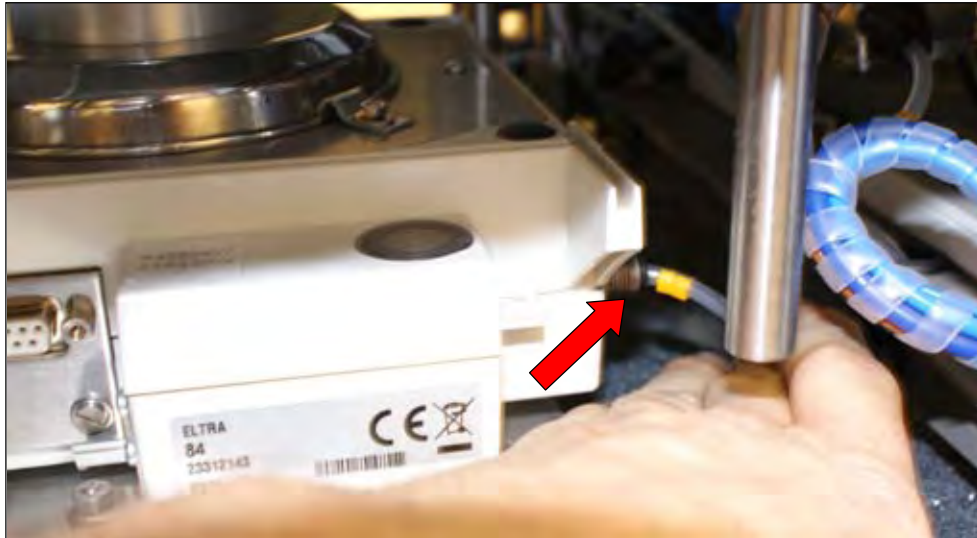
Fig. 3.8.5: LHS – Disconnecting purge tube of the balance
