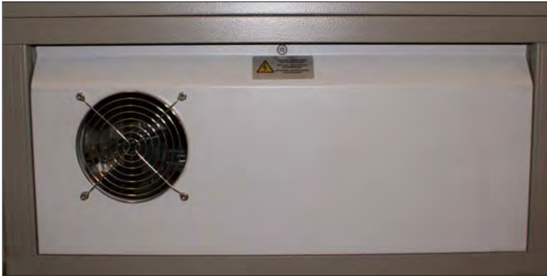
Fig. 1.14: LHS – Lower side panel with notch for exhausting air tube
