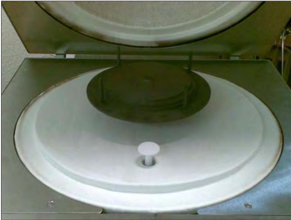
Fig. 1.1.: Carouseladaptor – inserted at the lower heating element
