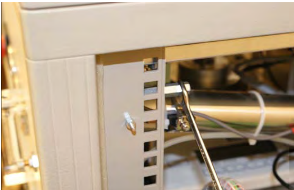
Fig. 3.7.1: LHS/RHS – Unfasten of front metal plate
