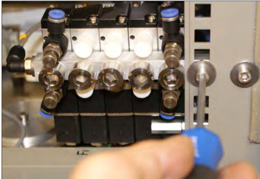
Fig. 3.8.3: LHS – Unscrew manifold
