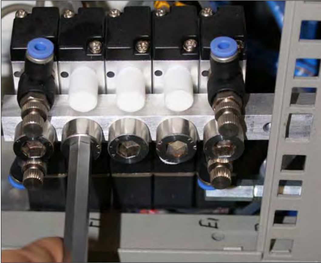
Fig. 3.2.5: LHS - Removal of the valve from the metal rail
