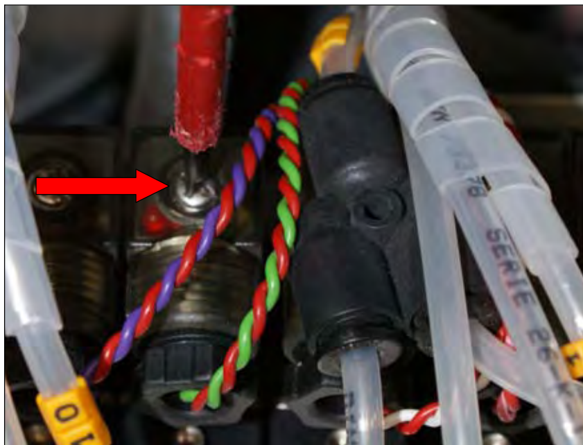
Fig. 3.2.4: LHS – Unfasten the power supply of the valve
