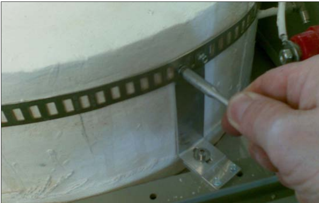
Fig. 3.16.6: Loosening the steel strap around upper heating element
