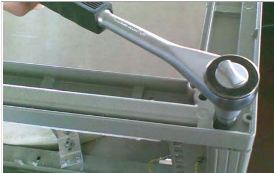
Fig. 3.16.3: TS – Removing bolts attaching the cover frame
