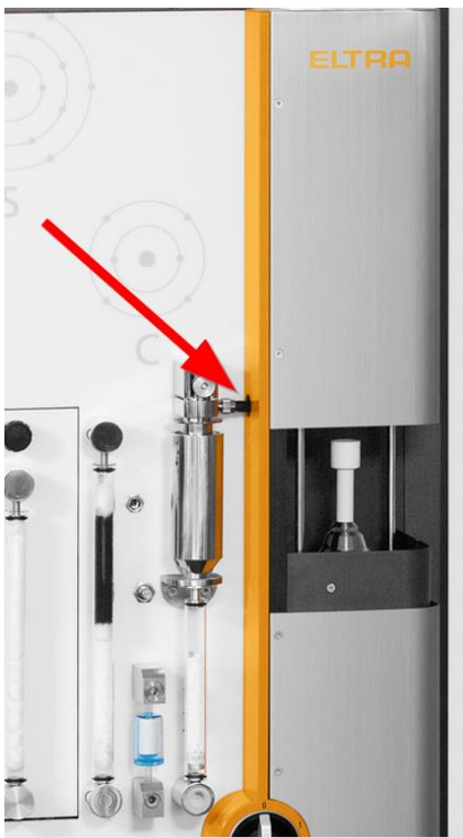
Fig. 72: Hose connection dust filter / furnace
