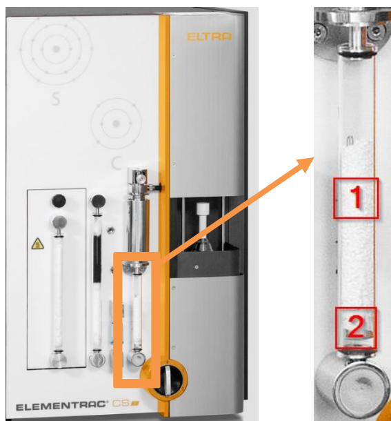
Fig. 56: Moisture trap replacement
