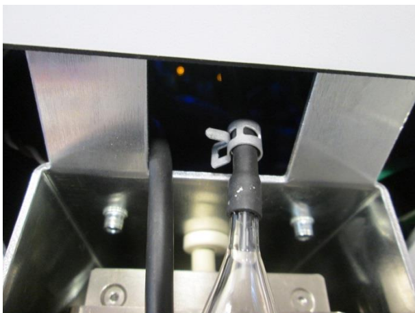
Fig. 46: Removing the clamp on the quartz tube of the catalyst furnace
