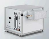
Determination of hydrogen using the heat extraction method is a special requirement for the characterization of steel, steel alloys, copper and other metals. **ELTRA's H-500 is designed for the rapid and accurate determination of hydrogen in these materials.**
