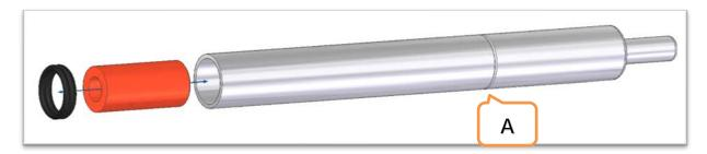
If the tool is prepared as described, it can be used to push the filter into the glass tube until the marking is reached (A).
