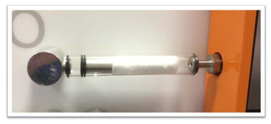
The gases from the furnace enter the dust trap from the right. The wool blocks most particles. Those particles which pass the wool are then blocked by the filter.
