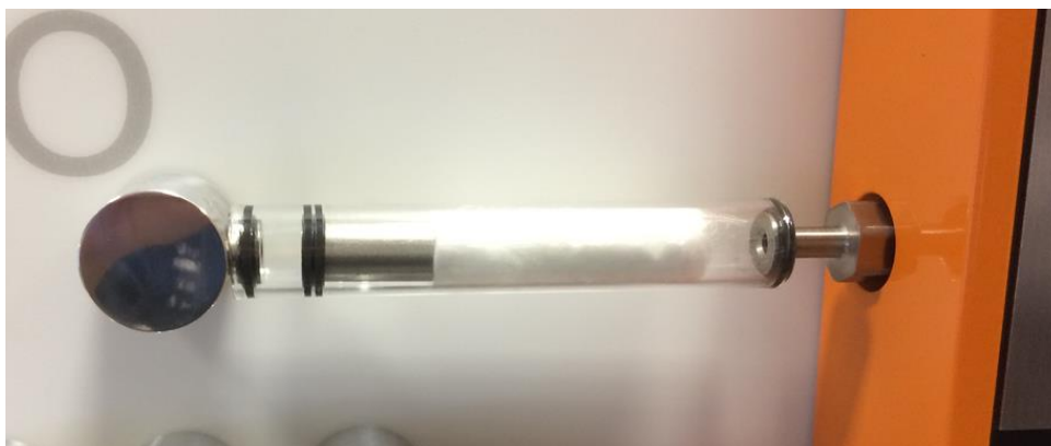
Fig. 5: Dust filter with sinter filter
