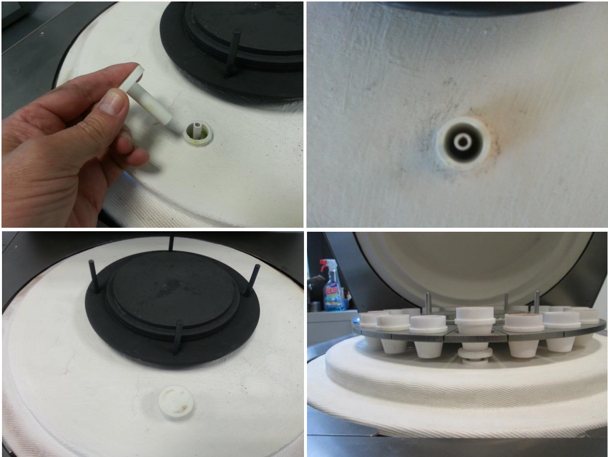
Fig. 4: Placement of the balance pedestal (inside furnace)
