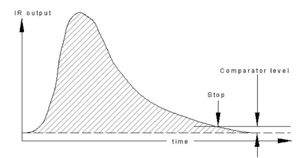
The comparator level is an artificial zero level, which rests just above the true zero level (base line) of the combustion curve diagram. If the detector signal level descends to the comparator level before the end of the maximum analysis time, then the analysis is finished. If the detector signal did not rise or already descended before the end of the minimum analysis time, the analysis will be continued until the minimum analysis time is expired.
