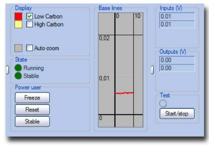
This window represents the automatic zero-regulation of the detectors' output signals. The controls of this process are available only for the power user. The detector's output signal in regulated and stable condition is taken as a reference zero level during analysis and is commonly called "*Base line*". The automatic zero adjustment of the detectors' output signals is commonly called "*Base line regulation*". See also <u>Theory: Base line</u>.
