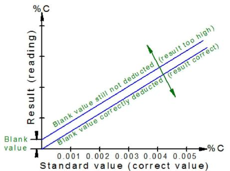
NOTE: In any circumstances, the appropriate actions must be taken, which exclude or reduce the blank value. For example, as pure as possible carrier gas, the good quality consumables, preheated crucibles or boats should be used. In case if it is not possible to exclude the blank value, the blank value determination procedure should be carried out. **Blank value determination procedure:**
