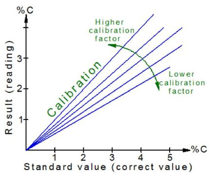
The calibration of the analyser is carried out using the standard samples only, i. e. the samples the concentration of the measuring element in which is known.
