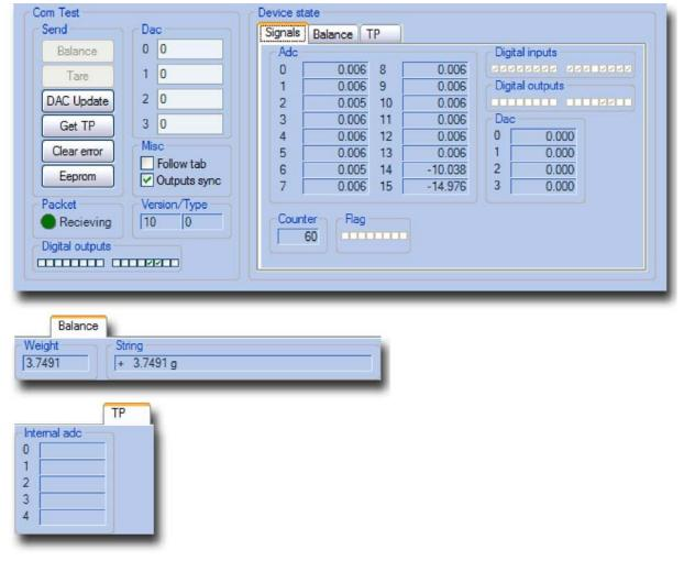
This window is used to check the communication and test the analyser (see <u>Theory</u>: <u>Controller</u>). It is available only for technician/service personnel!
