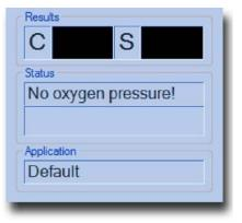
This window displays the analyses results, information on current phase of analysis procedure, error messages, current analysis information (sample weight, sample ID etc.) and current application name.
