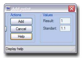
The new point for multipoint calibration for selected measuring channel can be entered in this window (see <u>Window: Multipoint calibration</u>).
