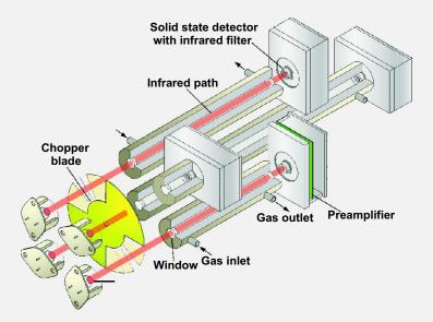
The lengths of all four cells can be individually optimized to obtain maximum precision for the target analysis levels of each customer. Each of the cells can be installed with infrared absorption lengths ranging between 1mm and 320mm.
