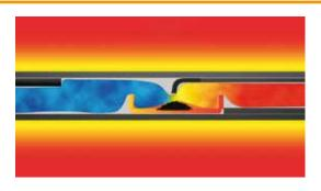
The horizontal resistance furnace of the CS-580 | CHS-580 is equipped with a ceramic combustion tube and silicon carbide heating elements. Full electronic control of the furnace ensures maximum service life of the components, including current limitation during heating-up. A sensor monitors ambient temperature and provides data for automatic reference point compensation of the thermo control, ensuring that the furnace temperature remains unaffected by fluctuations of the ambient temperature.
