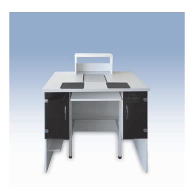
Professional Weighing Table is intended for the use with microbalances and analytical balances. It is incorporates an independent anti-vibration table with a stone table top. This solution eliminates possible vibrations and significantly shortens balance stabilization time.
