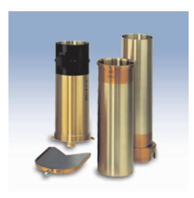
This kit is designed for determination of density of cereals. Measurement of cereal density in loose state is performed with application of precise balance series WPX 4500/G and density kit for cereals. Density determination result is calculated automatically by balance software (in accordance to tables containing cereal density).
