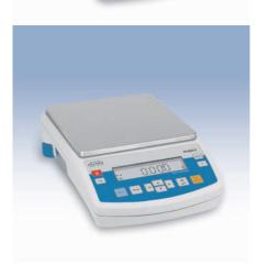
Pharmaceutical balances series PS are equipped with 12 key front panel and LCD backlit display. Pan dimension is this series is 195×195 or 128×128 mm with a glass shield over the weighing pan which protects the load against possible breeze. Each balance has RS 232 and additional display outputs as standard.
